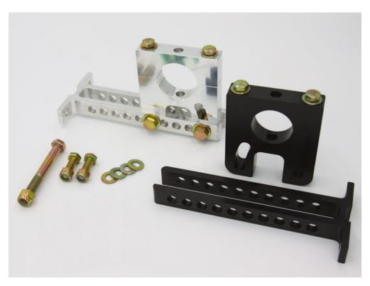
The Billet Upper Adjustable Seat Mount comes with all necessary hardware, including those needed to attach the seat mount to your aluminum racing seat and the hardware needed to comply with NHRA rules. The Billet Upper Adjustable Seat Mount includes the crossbar clamp, which attaches to the roll cage's seatbelt crossbar, and the adjuster tee, which attaches to the seat and crossbar clamp.
