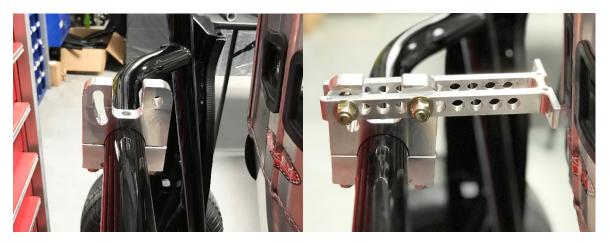
Rotating the crossbar clamp 180 degrees to the top will come in handy if your vehicle's crossbar is lower, or the height of your seat is higher. We realize not every seat mount arrangement is the same, and our Billet Upper Adjustable Seat Mount reflects that thought. It is truly designed and built to fit a wide variety of seating solutions.
