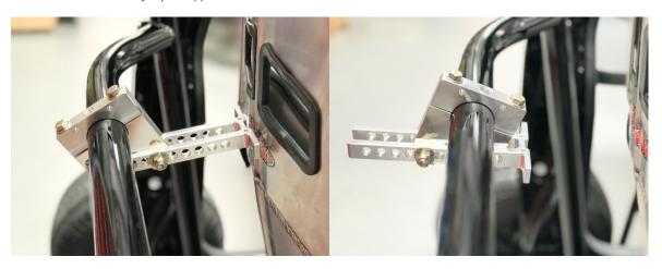
Depending on where your seat is mounted, and the location of your crossbar, those two measurements will dictate how you mount the crossbar clamp. The crossbar clamp, depending on how you mount it, provides almost 5 inches of adjustment. With the crossbar clamp, you can get the seat as close as 17/8", and as far away as 6".
