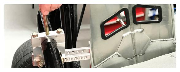
To comply with NHRA rules, we include a Grade 8 bolt and nut to attach the mount to the crossbar. (left) According to NHRA rules, one bolt must go through the crossbar and crossbar clamp to be NHRA-legal.(right) Furthermore, the Kirkey seat we are using here is reinforced in the area needing drilled for the FFP Billet Upper Adjustable Seat Mount.
