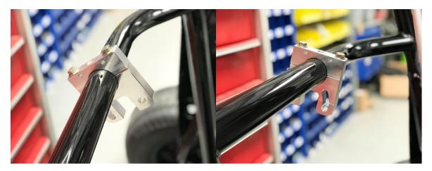
Here are just two examples of how to mount the crossbar clamp. Remember, the crossbar clamp can be rotated and flipped in whatever manner works for your application.
