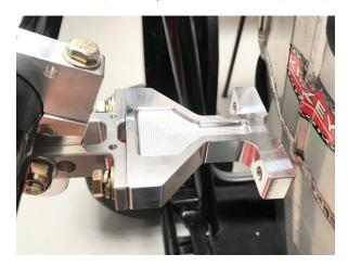
Once attached to the Billet Upper Adjustable Seat Mount, you can fine-tune the Billet Upper Adjustable Seat Mount Extension's location as it relates to the seat. It's easier to adjust the Billet Upper Adjustable Seat Mount's adjustment tee to fit your application.
