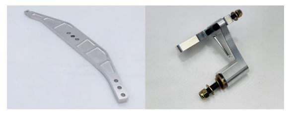
The throttle pedal is sectioned off by itself in the box when you receive the pedal assembly. It uses a throttle pedal stop and hanger that attach it to the main structure. This is the throttle pedal stop and hanger (Right). It attaches to the pedal, which attaches the pedal to the main structure.
