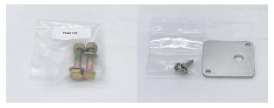
Additional hardware for the throttle pedal is for the pedal pad installation and for the throttle cable firewall bracket.
