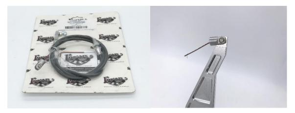
With all the different throttle cable lengths and applications, we do not include one with our pedal assembly. However, this Lokar cable is an example of what we recommend. The Lokar TC-1000U36 is a 36" cable, which may work for some of you, while others may need a longer or shorter throttle cable. The throttle cable attaches to the top of the throttle pedal using the attached clevis, goes through the firewall, and then attaches to your car's throttle linkage.
