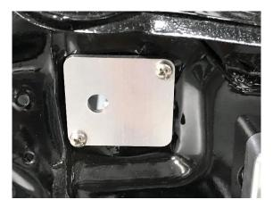
The throttle cable firewall bracket uses the factory clutch cable opening in the firewall. There is already one hole that is used to secure the factory clutch cable, so you must make another hole for the throttle cable bulkhead. This picture was taken facing the firewall.
