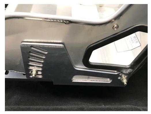
If you would like to move the seat to the highest point the side seat mount will allow, drill the rear hole in the seat at the lowest point. This will allow the seat to sit up higher to fit the comfort and safety of the driver.
