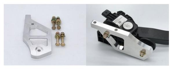
We made this bracket to bolt a Ford Performance Control Pack Electronic Throttle Control pedal to our Patented Pedal Assembly. Our bracket attaches to the Control Pack pedal, and then the bracket is bolted to the pedal assembly. This bracket will also work with a factory 2005-2014 Mustang GT throttle pedal, as well. The  $4-28 \times 1 \%$  bolts are to mount the bracket to the main structure, while the  $4-28 \times 1 \%$  are to mount your pedal to our bracket.
