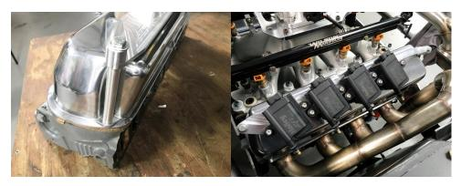
Here is a close-up of the spacer, bolt, and washer arrangement for the Small Block Ford Smart Coil Mounts. Our Small Block Ford Smart Coil Mounts use the top bolt holes on each side of the head/valve cover for attachment. On our own Ultra Street car, this is the finished product. Our Smart Coil Mounts can also be flipped side-to-side to accommodate front or rear breather fittings. We have these Small Block Ford Smart Coil Mounts on everything from ground-pounding hot rods to full-on race cars.
