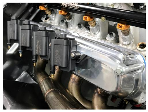
In this picture, on our shop car, our Smart Coil Mounts use Holley Smart Coils. However, most Smart Coils feature the same bolt pattern, so our Smart Coil Mounts are compatible with most aftermarket LS -style coils.
