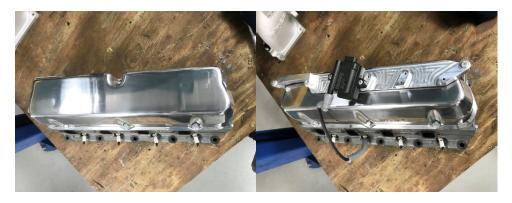
Here we have a classic GT-40P head with a standard valve cover installed. This is one of our display pieces we take to shows and events. To install the Smart Coil Mounts, simply use the two provided spacers, the longer bolts in the hardware kit, a washer for each bolt, and the Smart Coil Mount itself. Here is where you will need your 7/16" socket and ratchet, or wrench.
