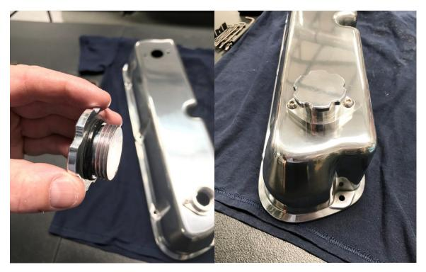
To finish the Oil Fill installation, make sure the O-ring is on the cap before threading it on. We add a very slight coat of grease to the threads to properly lube the O-ring. Just like that, you are done with the Oil Fill installation. Our natural finish Oil Fill looks great on polished, or chrome valve covers.
