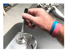
Then, using a Sharpie, trace the inside diameter of the Oil Fill's opening, and use the step bit to drill out the hole. Then follow up with a burr bit to clean up the hole of any rough areas or shavings. As a reference, the Oil Fill's opening is 1.17", but for many people, tracing the inside diameter while marking the valve covers for the bolt holes will be the easier route. Once everything is drilled and deburred make sure to clean out the valve cover, getting rid of all shavings.
