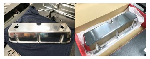
This is our display valve cover for which we use to showcase our Bolt-On Oil Fill and AN Fittings at the track. As you can see, we already have provisions for both products. This gives you an idea of how your valve covers should look after the drilling process. However, let's say your valve covers lack these provisions. We can still guide you through the installation process.
