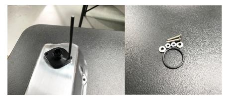
Once you have decided where to mount the fitting, use a punch to mark the hole location for the hardware. Then use a Sharpie to trace the hole for the opening. The -10 AN Fitting hole is roughly half an inch, while the -12 Fitting hole is roughly 5/8-inch. Hardware for the AN Fittings is included, which entails buttonhead Allen bolts, rubber bonded washers, two nuts, and an O-ring.
