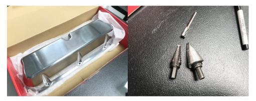
If you are starting with a valve cover without any grommet holes or PCV provisions, you will have to make your own. A couple tools you will need to drill new holes into your valve covers are obviously a drill, a step bit (Left and Right), and a burr bit (Top). You will need to make sure these bits are for aluminum. You can also use a hole saw. Whatever method you are more comfortable with will work. We are just giving you an idea of how we do it.
