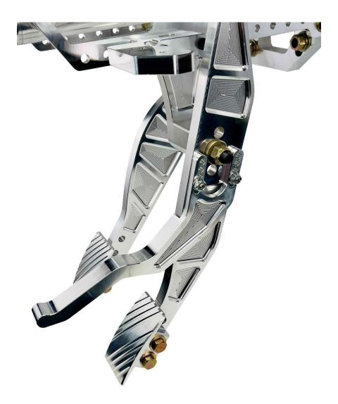
FFP Customs is always looking to improve the pedal assembly to accommodate all driver needs while still maintaining a smooth and headache free installation. The FFP toe hook allows drivers to have full control of their throttle when using a solid linkage/cable. This lets the driver manually close their throttle body(s) with the movement of their foot. The installation of the toe hook is simple, using only two 10-32 bolts, two 10-32 nylock nuts, and two 10-32 washers.
