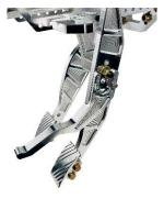
The photo above shows how the optional Throttle Toe Hook is mounted to our pedals using the 2 small holes in the middle of the pedal. This feature is useful in applications where the driver needs to be able to close throttle blade using a push-pull style cable or solid linkage.
