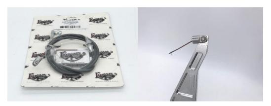
With all the different throttle cable lengths and applications, we do not include one with our pedal assembly. However, this Lokar cable is an example of what we recommend. The Lokar TC-1000U36 is a 36" cable, which may work for some of you, while others may need a longer or shorter throttle cable. The throttle cable attaches to the top of the throttle pedal using the supplied clevis, goes through the firewall, and then attaches to your car's throttle linkage.
