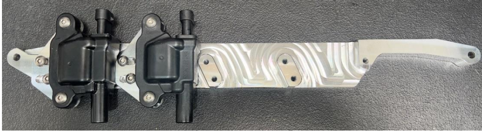
Figure 2 Passenger Side Coil Mount with 2 LS3 style coils mounted. Repeat for remaining coils.
