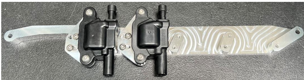
Figure 4 Driver Side Coil Mount with 2 LS3 style coils mounted. Repeat for remaining coils.
