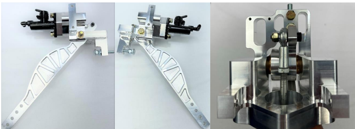
The clutch master cylinder uses this spacer and studs to attach it to the clutch pedal.
