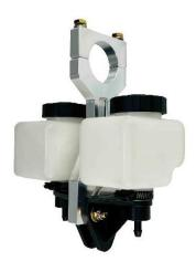
The main structure/brake pedal assembly includes this reservoir mount for the brake master cylinder. This mount is designed to use the roll bar running behind the dash, but if you don't have that, the reservoirs still need to be mounted above the master cylinder for proper operation as they are gravity fed.
