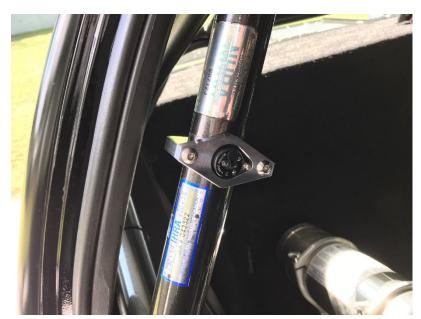
Installation of an FFP Customs Wireless LED Roll Bar Light Mount literally takes minutes to accomplish. Using a 5/32 Allen wrench or socket, simply insert the LED bulb into the flat part of the mount, fit the other half around the roll bar, and then tighten the two together. It really is as simple as that.
