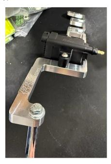
Here is a close-up of the spacer, bolt, and washer arrangement for the Small Block Ford Smart Coil Mounts. Our Small Block Ford Smart Coil Mounts use the top bolt holes on each side of the head/valve cover for attachment. These mounts can be used with front, rear, & staggered mounted valve cover fittings.
