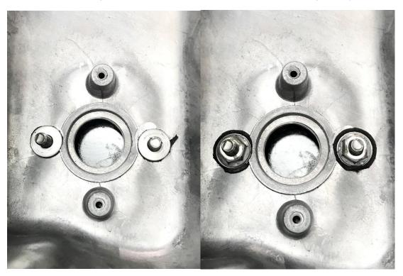
This is how the rubber-bonded washers should look. This is looking into the valve cover from inside. Use a ratchet with a 7/16" socket and a 5/32 Allen wrench to attach the Oil Fill to the valve cover. The rubber-bonded washers must be flat against the valve cover. We had to do a little clearance work to get ours flat against the valve cover's surface.
